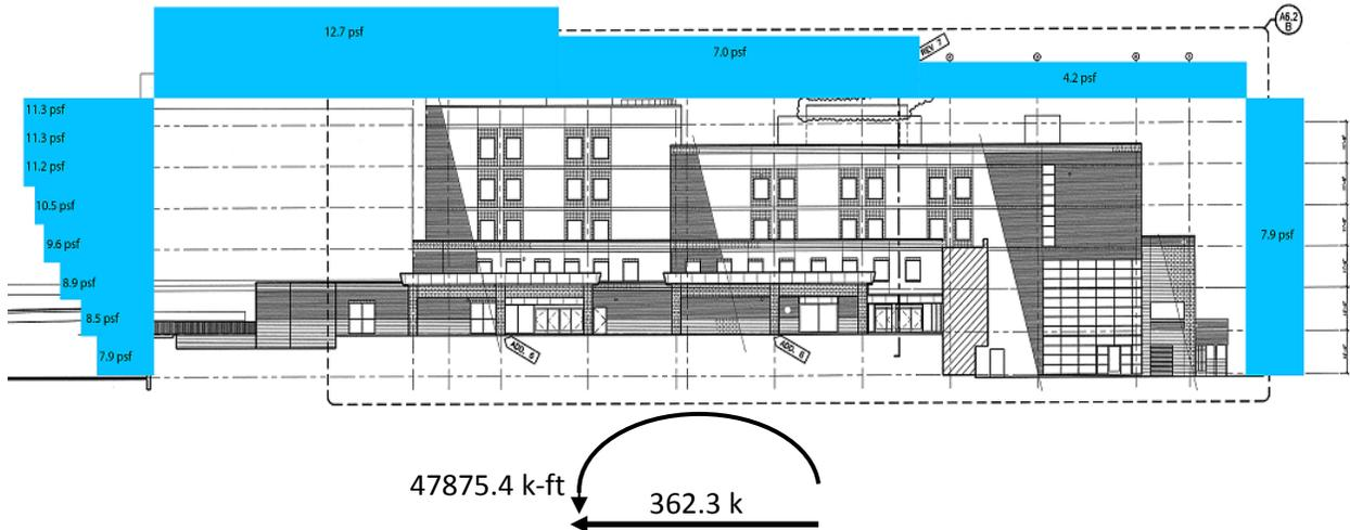
Figure 5: Wind Loading – East to West
