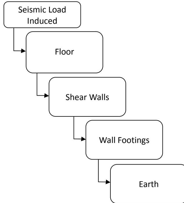
The seismic load will travel through the floor and follow the stiffness to the shear wall. The shear wall will directly transfer its load to its base, the wall footings and then release the load to the earth.
