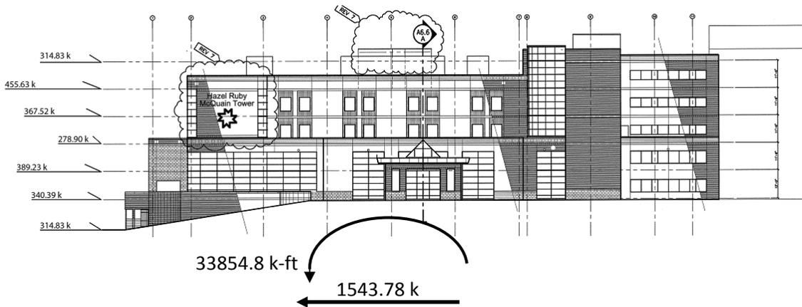
Figure 7: Shear Wall Group 1 Loaded in X Direction
