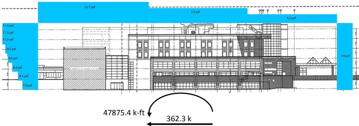
Figure 6: Seismic Loading
