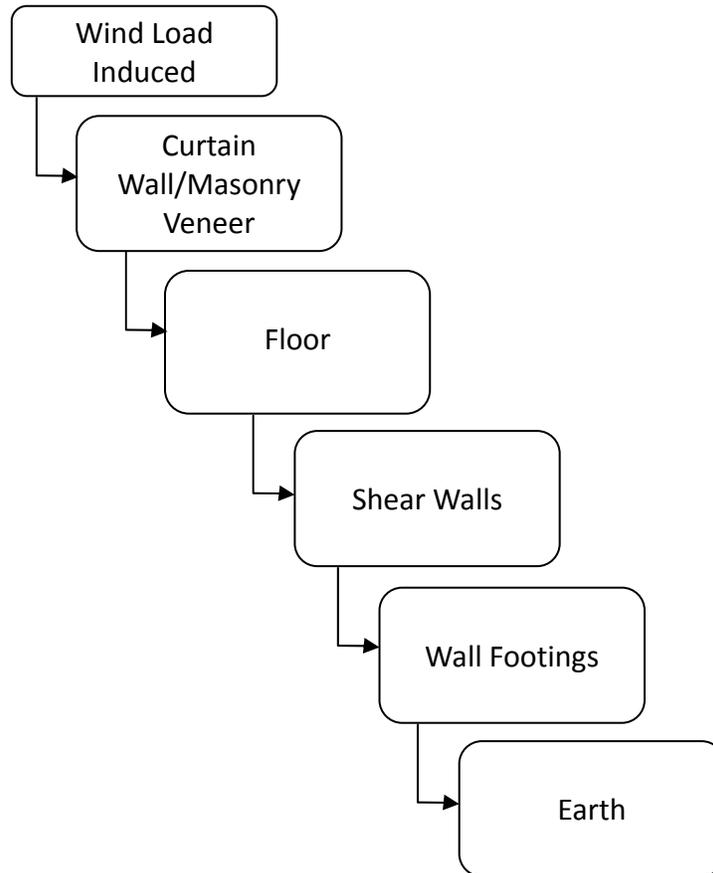
The load induced by the wind will travel through the curtain wall or the masonry veneer, travel through the floor. The load will then follow the stiffness to the shear walls (stiffest structural member of the Hospital), and the load is directly transferred downwards to the footings and then to the earth.
