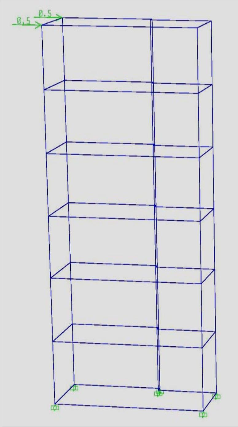
Figure 9: Shear Wall Group 3 Loaded in Y Direction
