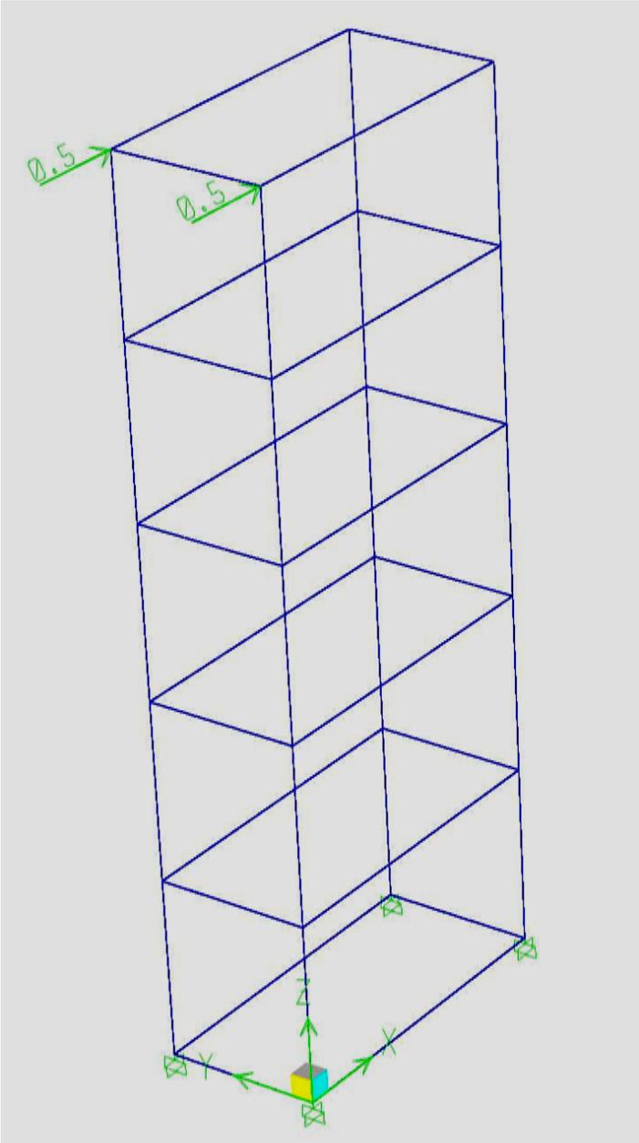
Figure 8: Shear wall Group 2 Loaded in X Direction
